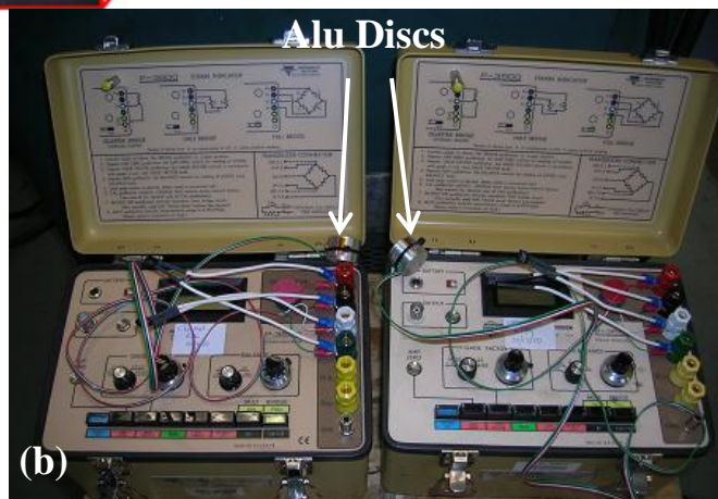
Figure 4-1: Aluminum disks with attached strain gauges used in measuring contact force during embossing (a), and bridges used to convert strain gauge signal (b)
